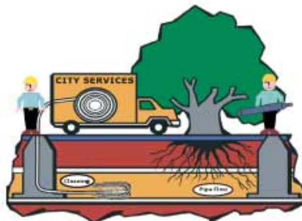
Cleaning the line
